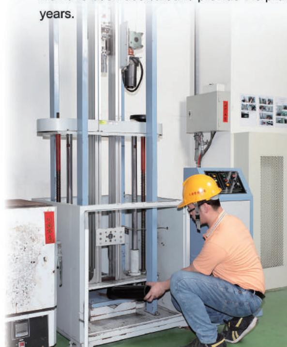
耐落錘測試實驗裝置 Falling hammer resistance device
