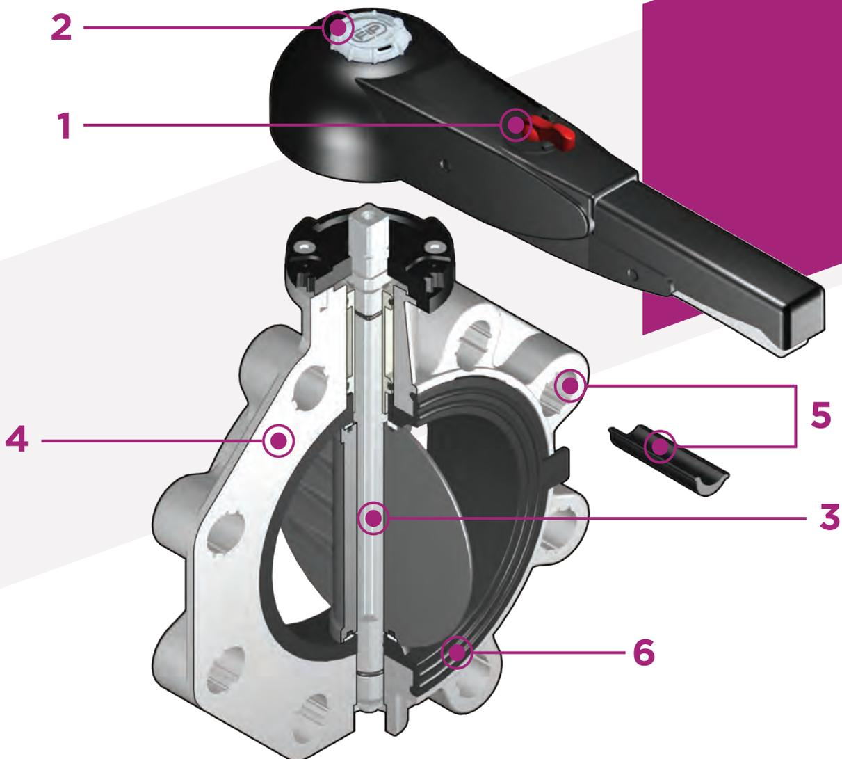
**1 Ergonomic handle in HIPVC** equipped with **locking and unlocking device, release, quick operation and graduated adjustment** in 10 intermediate positions (DN 40÷200). The operating range, starting from the first few degrees of valve opening, also guarantees extremely low pressure drops.
