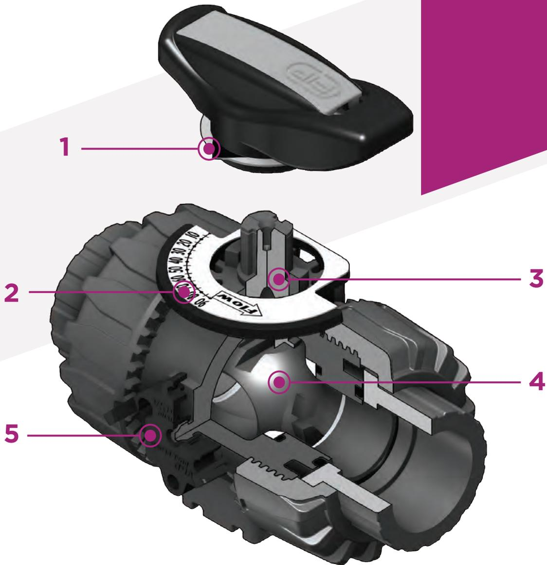
**1** HIPVC ergonomic multifunctional handle with **position indicator** and removable key to **adjust the ball seat carrier**
