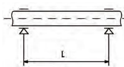
The installation of thermoplastic pipe systems requires the use of support clips to prevent flexing and the resulting mechanical stresses. The distance between the clips depends on the pipe material, SDR, surface temperature and the density of the conveyed fluid. Before installing the clips, check the distances reported in the table below, as provided for by guidelines DVS 2210-01 for water pipes.
